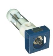
**Spectra Pump Model: S08B04** used to dose 25 l/h of chemical. The pump liquid end is flanged directly to an SEW helical gear reducer, LP adaptor and TECO 0.37 KW single phase motor. The rotating components of the pump are hastelloy and the casing is manufactured from RCH1000.
